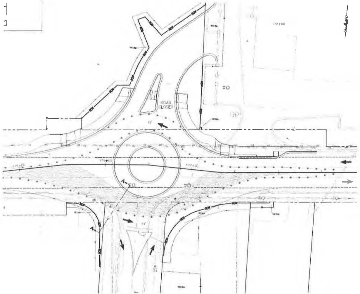
Figure 16-3 Renninger Roundabout Construction - Stage 2a
