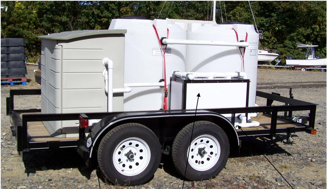
Connection to pressure washer Bag filter tank Backwash line connection
