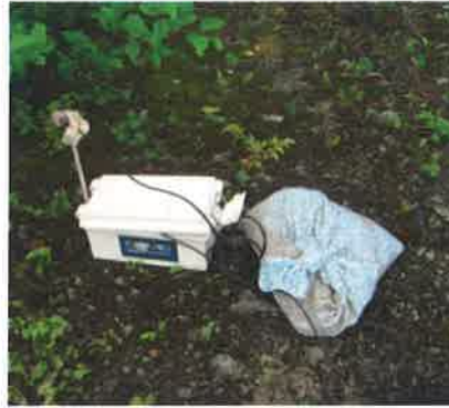
Figure 2. Left. Installing triaxial geophone in ground.
