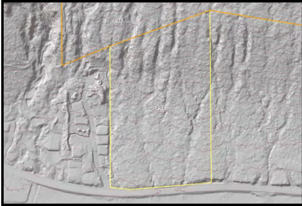
Figure 2 - Hillshade with 10 foot contours. Showing the deep stream gullies in the NW corner and the lack of deep gullies in the NE corner.
