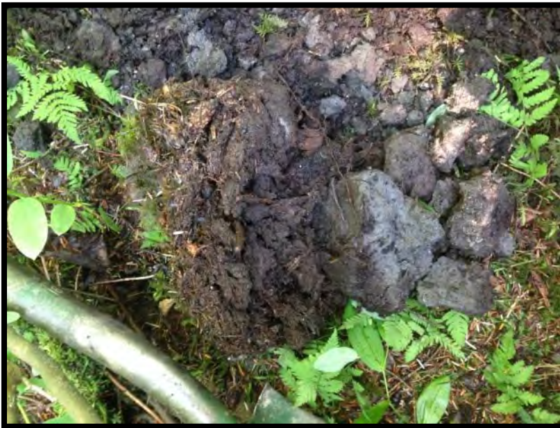
Photo 2 - Four inches of well-drained organic matter over a sandy silt loam at sample pt. #1.
