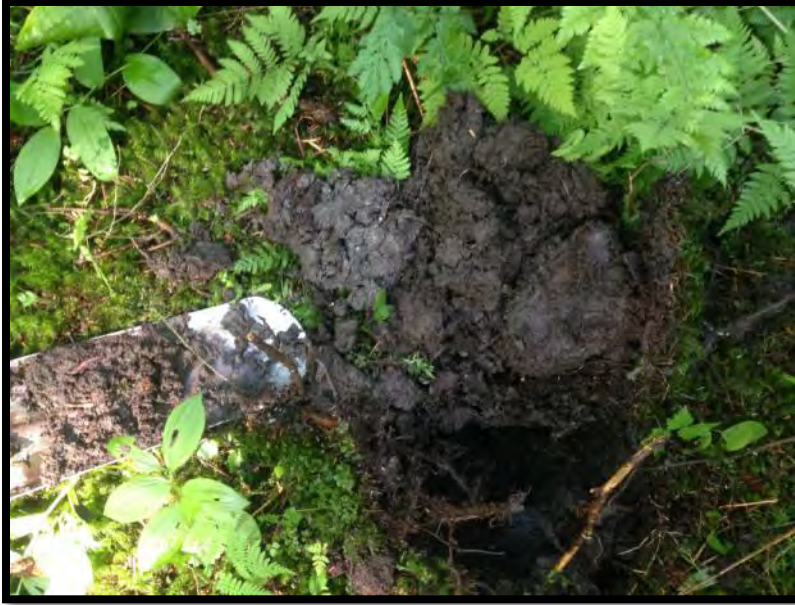
Photo 1- Wadleigh Series soil with 8 inches of saturated peat over a dense glaciomarine sediment of sandy silt loam at sample pt #2.
