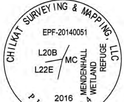
PRIMARY MONUMENT 2.5" x 30" ALUMINUM PIPE WITH 3.25" DIAMETER ALUMINUM CAP WITH CLEAR DEEP 1" MAGNET AT THE BASE
