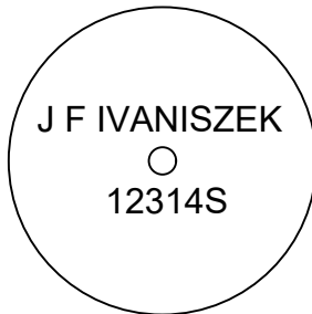
5/8" x 36" REBAR WITH RED PLASTIC CAP
