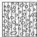
SMg SILTY SAND WITH GRAVEL
