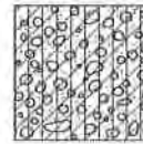
(SC-SM)g SILTY, CLAYEY SAND WITH GRAVEL
