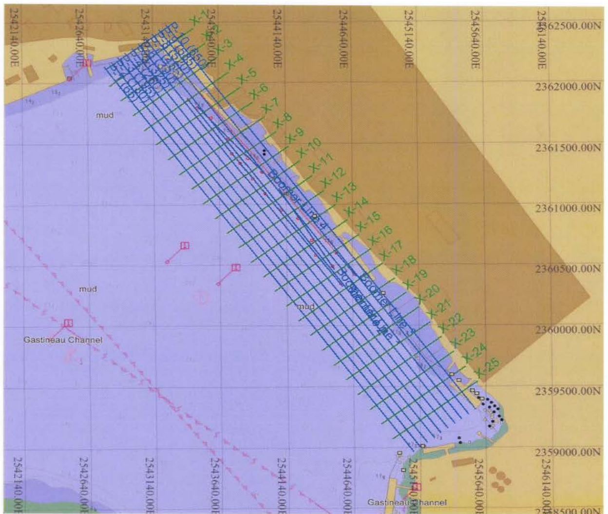
Figure 2: Proposed SBP/Boomer Line Plan.
