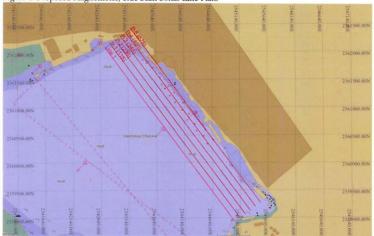
Figure 1: Proposed Magnometer/Side Scan Sonar Line Plan.
