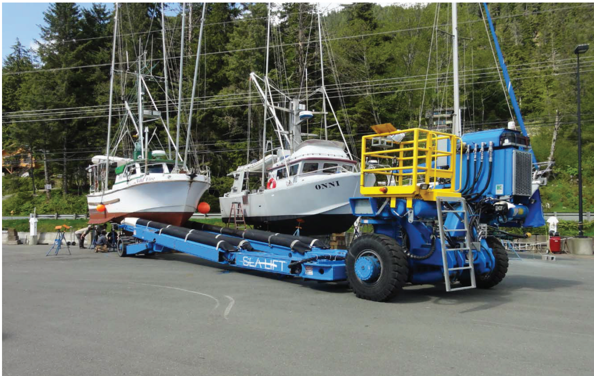
PHOTO 14 - SIDE VIEW OF SEALIFT TRAILER AS IT DISENGAGES FROM BOAT (051518_2526)
