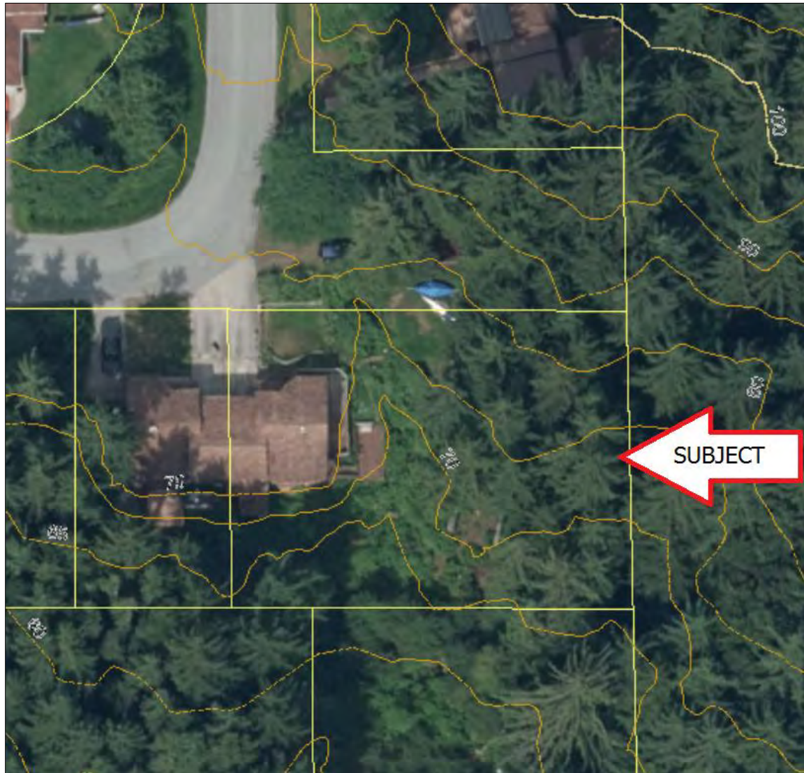
Aerial topography -- Contour lines at 5' intervals
