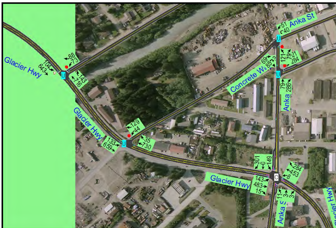
Figure 15: Projected 2027 P.M. Peak Hour Turning Movement Volumes for Alternative 2
