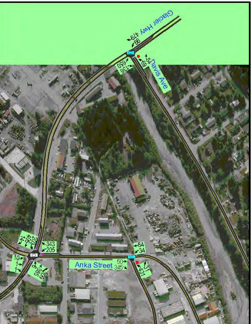
Figure 6: Projected 2027 P.M. Peak Hour Turning Movement Volumes
