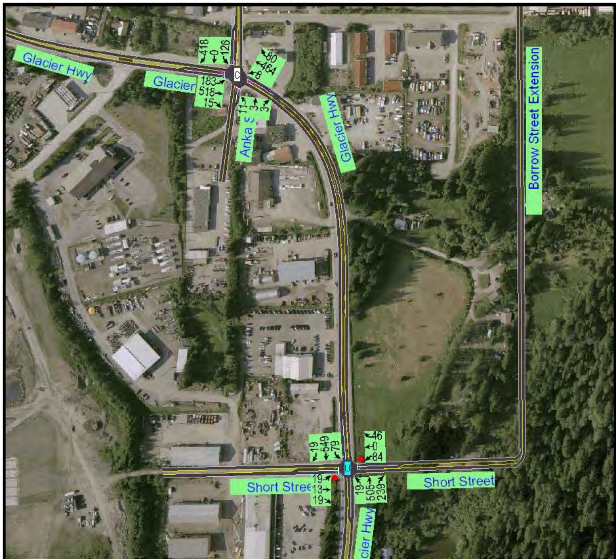
Figure 17: Projected 2027 P.M. Peak Hour Turning Movement Volumes for Alternative 4
