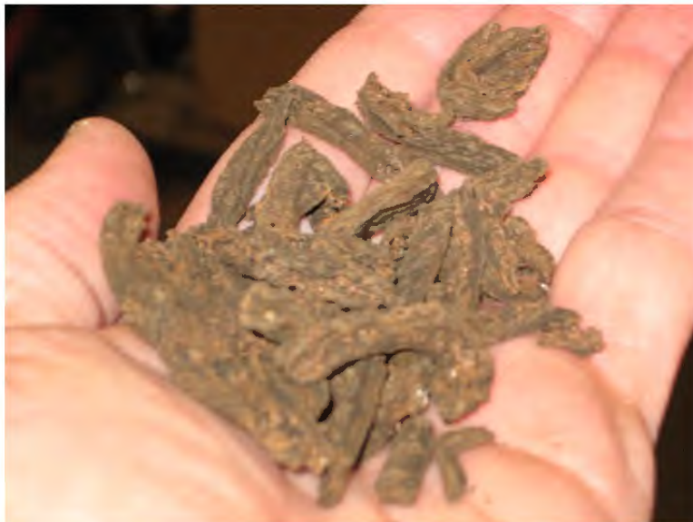
FIGURE 2 Dried Biosolids Product from a Belt Dryer (courtesy of Kruger)
