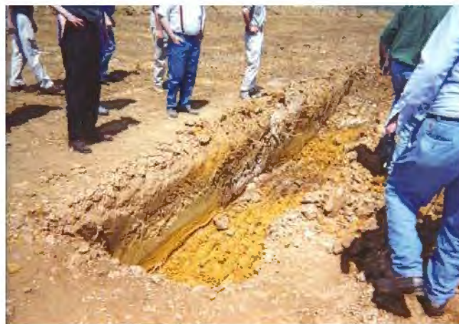
FIGURE 1 EXCAVATED CROSS-SECTION OF BIOSOLIDS TRENCH
