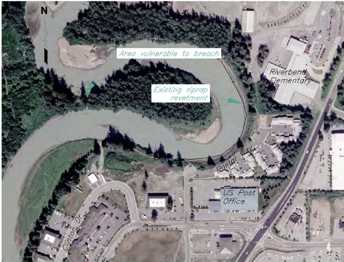
Figure 2: Existing streambank protection and area of concern near Postal Way and Clinton Drive
