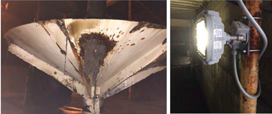
Left to right: JDTP surface impeller condition prior to replacement; new interior LED lighting
