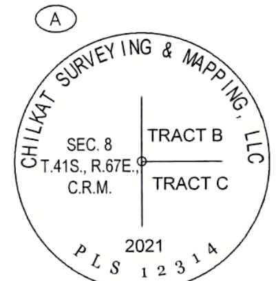
PRIMARY MONUMENT 2.5" x 30" ALUMINUM PIPE WITH 3.25" DIAMETER ALUMINUM CAP WITH CLEAR DEEP 1 MAGNET AT THE BASE
